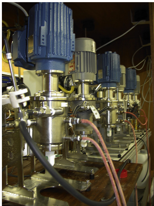
Fig. 3. Experimental setup of CCS devices. Six devices in line are used for the ELLE of Pgl, a seventh CCS for the back-extraction is positioned further backwards in the hood.
